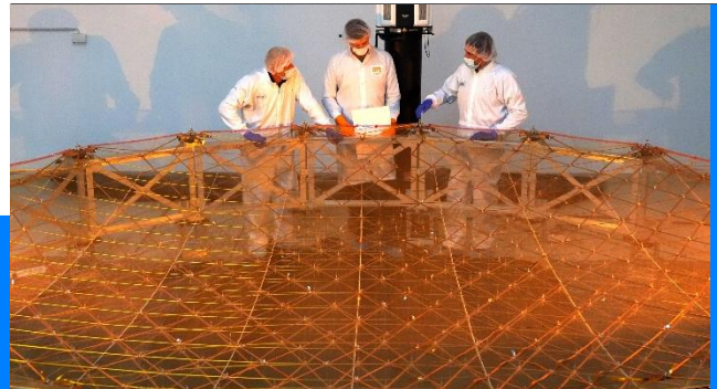
5 m large deployable reflector surface with HPtTex-USM-mesh under RF testing at Airbus Germany
