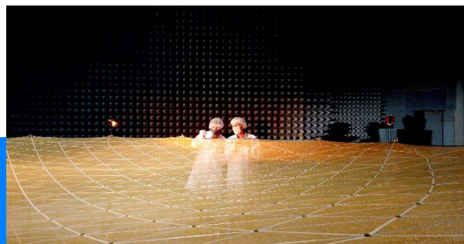
5 m large deployable reflector surface with HPtexas-USM-mesh under RF testing at Airbus Germany
