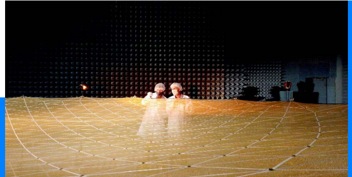
5 m large deployable reflector surface with HPtEX-USM-mesh under RF testing at Airbus Germany
